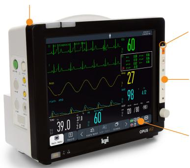
**'Smart Sensor'** adjusts screen brightness automatically to maintain high legibility
